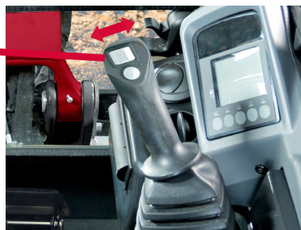
2 Proportional PTO control lever
